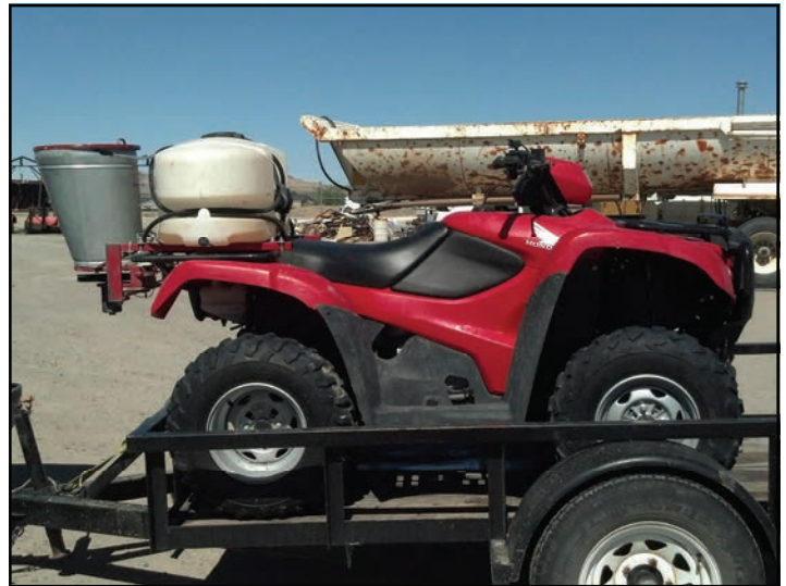
Figure 1. Quad runners equipped with Herd seed spreaders and 12 or 25 gallon liquid spray tanks.
