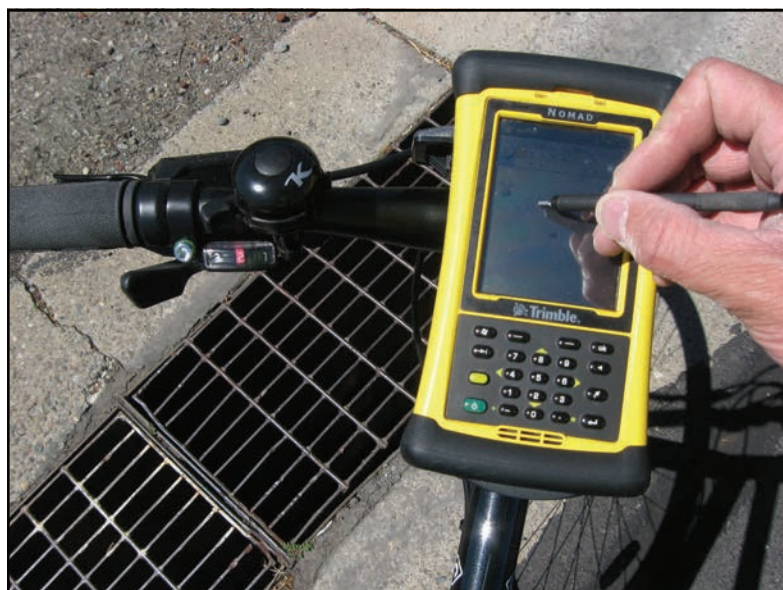
Figure 2. Hand-held mobile GIS data collection device secured to the bicycle handlebars.
