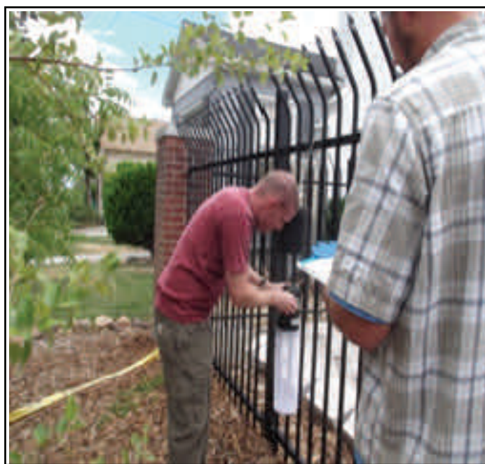
Figure 1. IHS staff members setting up CO 2 traps in an urban location near the University of Nevada Reno.
